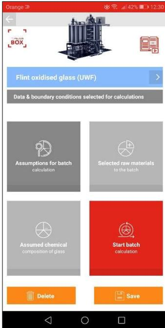
**Step 3. Screen 3** contains data and boundary conditions for the desired calculations: **Assumed chemical composition of glass**, **Assumptions for batch calculation**, **Selected raw materials**. To modify the chemical composition of glass, click the **Assumed chemical composition of glass** button.
