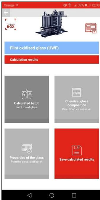
**Step 15.** The results of the calculation can be accessed on **screen 14**. After clicking the **Calculated batch** button, the total weights of all the raw materials can be seen for the defined amount of glass/batch/sand, which must be used to achieve glass with a defined composition.
