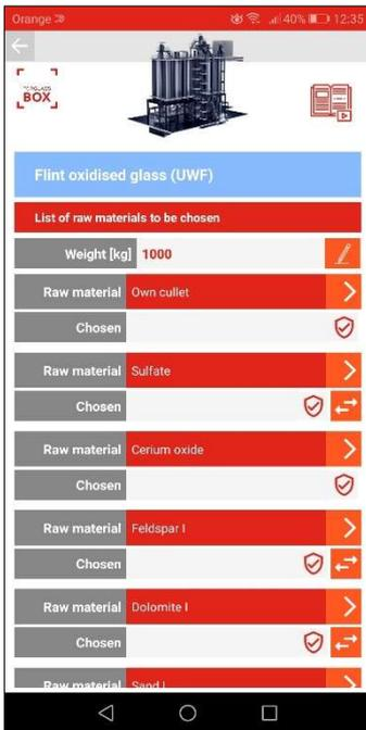
**Step 10. Screen 9** contains the list of raw materials selected for batch calculation. The user can modify composition of selected raw materials by clicking the > symbol to the right of the name of the material. Materials with alternatives have the additional ↔ button that can be clicked to reveal **screen 10**, which allows the user to choose alternate material.
