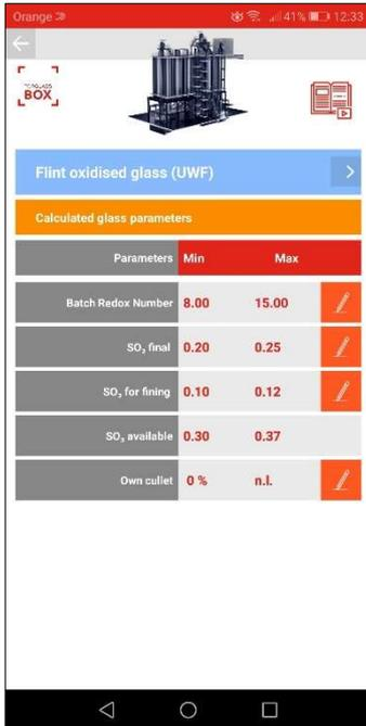
**Step 7. Screen 6** shows the assumptions for calculations, which can be edited by the user after clicking Edit button to the right of the selected set of values – see **screen 7**. The default values in each set are the most typical ranges of **BRN**, **final SO<sub>2</sub>** and **fining SO<sub>2</sub>** for the selected glass type. To save the changes, click the **Change** button; to discard the changes, click the **Back** button.
