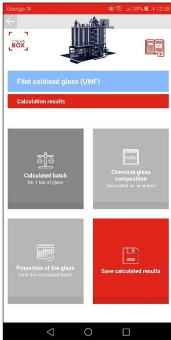
Step 17. The results of the calculation can be accessed on **screen 14**. After clicking the **Chemical composition of glass** button, next screen appears.
