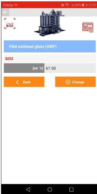
**Step 13. Screen 13** shows the window for editing composition of a sample of raw material selected for batch calculation. User can change the concentration of a component by entering the new value in the field and clicking **Save**. If you want to discard the changes, simply click the **Back** button. Similar operations can be performed for other components of the raw material.
