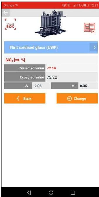
**Step 5.** After selecting the specific component of glass on **screen 5**, it is possible to change its concentration and the value for the maximum allowable deviation of those oxides (down  $\Delta-$  or up  $\Delta+$ ) in the glass. To save the changes, you must click the **Change** button. To discard changes, click the **Back** button.
