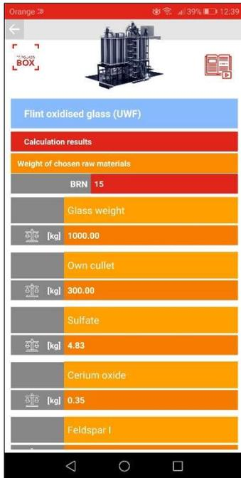
Step 16. **Screen 15** shows the batch calculated for the user-defined amount of glass/batch/sand.
