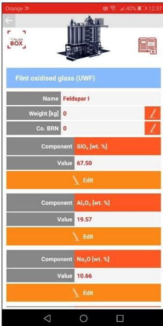
Step 12. **Screen 11** shows properties of a sample of raw material selected for batch calculation. User can adjust (change) the concentration of various oxides, according to the chemical composition of the raw material to be used in the batch. To make changes, click the ✎ icon next to the field you wish to edit.
